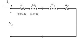
The equivalent impedance of the rotor circuit in parallel with  $jX_M$  is:
