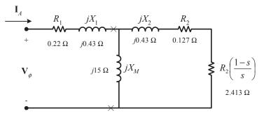
(a) The easiest way to find the line current (or armature current) is to get the equivalent impedance  $Z_F$  of the rotor circuit in parallel with  $jX_M$ , and then calculate the current as the phase voltage divided by the sum of the series impedances, as shown below.
