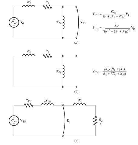
$$Z_{\rm TH} = \frac{jX_M (R_1 + jX_1)}{R_1 + j(X_1 + X_M)} = \frac{(j15 \ \Omega)(0.22 \ \Omega + j0.43 \ \Omega)}{0.22 \ \Omega + j(0.43 \ \Omega + 15 \ \Omega)} = 0.208 + j0.421 \ \Omega = 0.470 \angle 63.7^{\circ} \ \Omega$$
